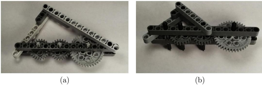
Figure 3: The approximate Pythagorean triples with sides  $\leq 14$  with (a) least absolute error (7-11-13) and (b) least absolute error for a hypotenuse slope of 1 (5-5-7). The hypotenuse in (b) is extended to provide more space for gears.
